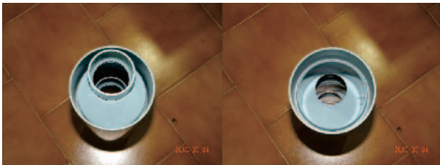
Fig.9 Eccentric-type reducer (110mm×63mm) in the main pipe of siphon system pipe-type fishway.
