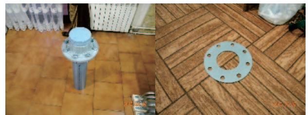
Fig.7 PVC flange, hand hole (left) and hand-made packing for flange (right). Packings for flange and hand hole do not work normally, but actually they are available for siphon system pipe-type fishway.
