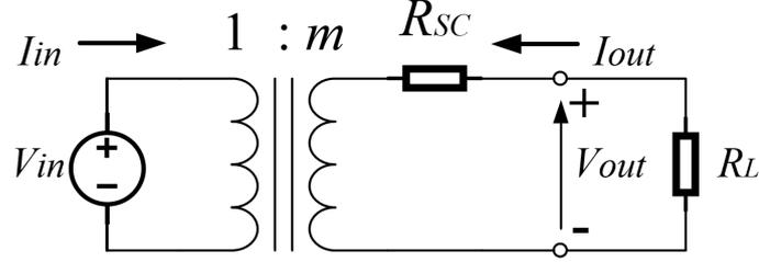
Figure 2.1: Four-terminal equivalent circuit model.
