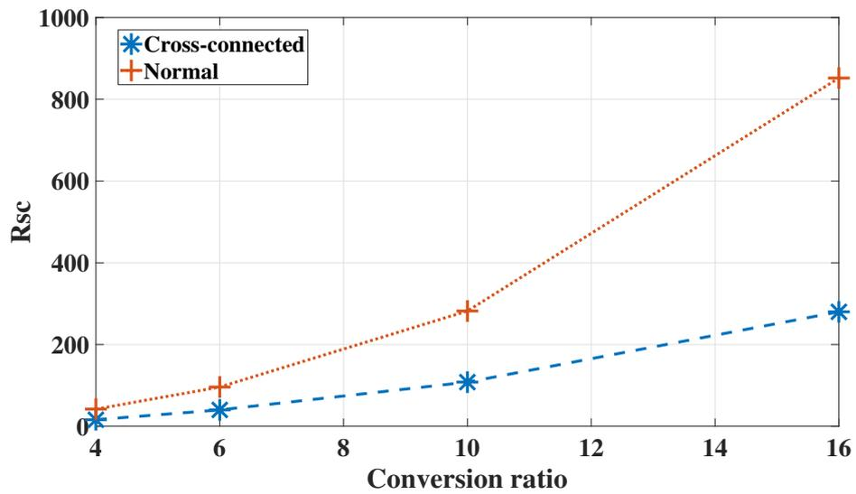
Figure 3.25: Comparison of  $R_{SC}$  of Fibonacci topologies.
