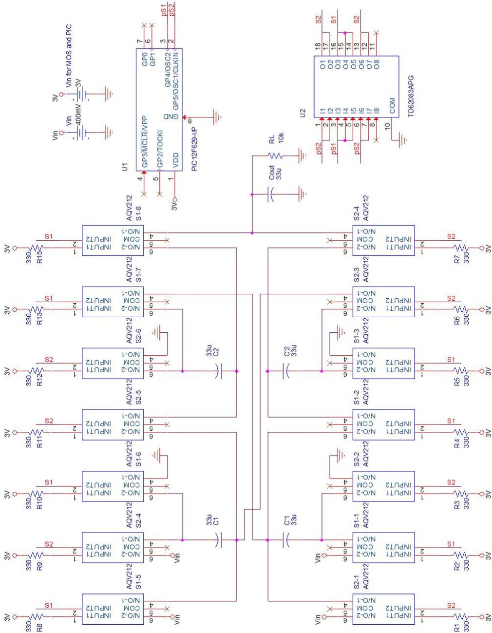
Figure 5.6: Experimental circuit schematic for cross-connected Dickson topology.
