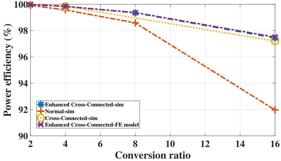
Figure 5.8: Comparison of power efficiencies of enhanced cross-connected Fibonacci topology.
