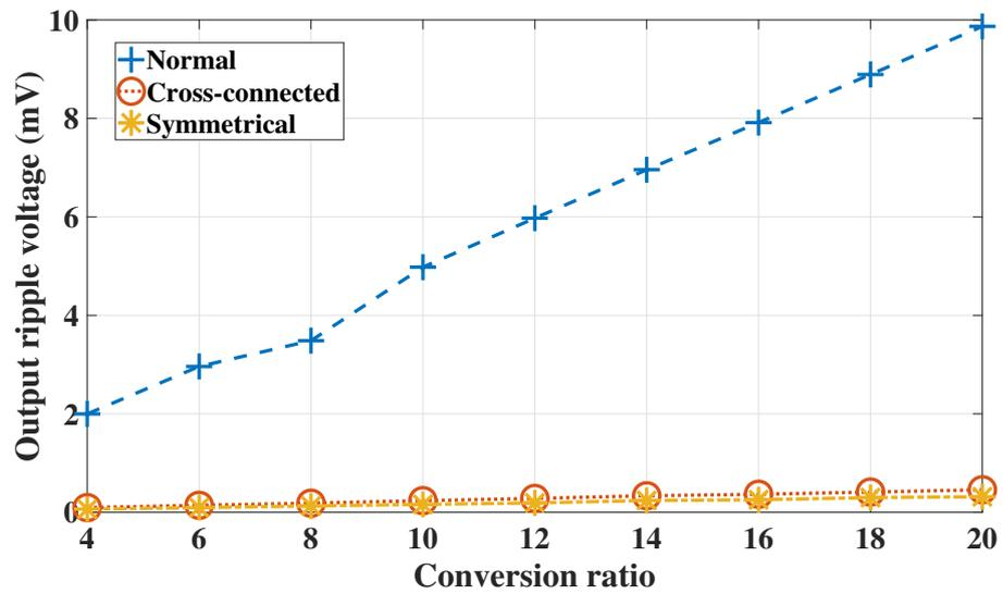
Figure 5.3: Comparison of output ripple voltages of Dickson topologies.
