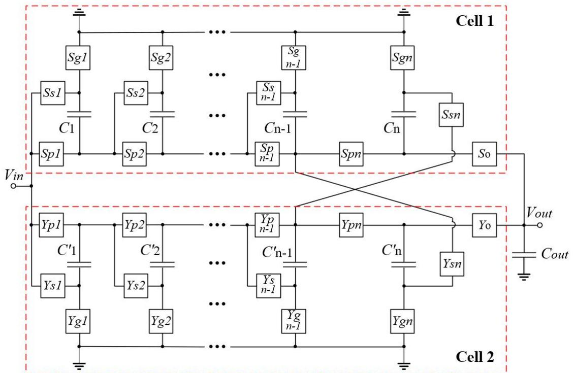
Figure 3.12: Cross-connected Fibonacci topology.
