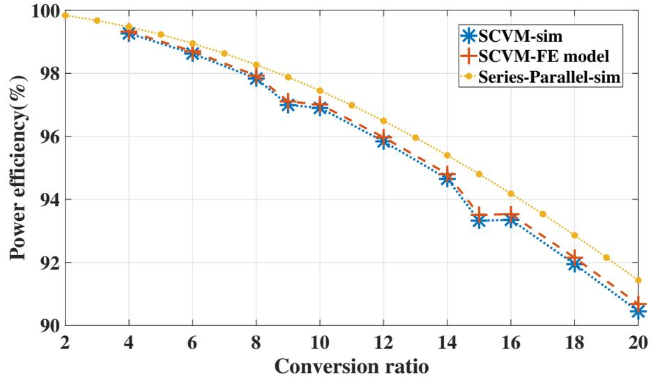
Figure 3.19: Comparison of FE model with simulation at different conversion ratios (SCVM topology).
