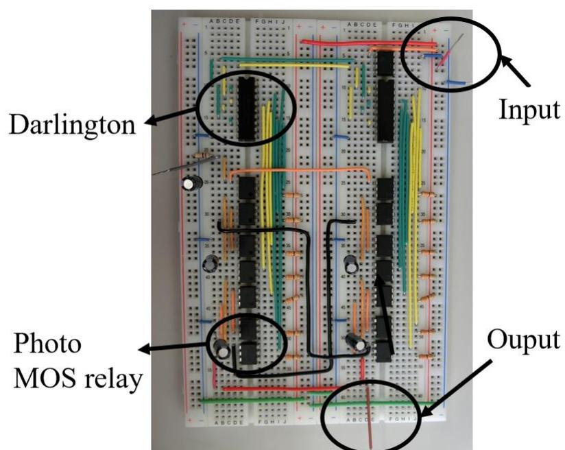
Figure 5.5: Experimental circuit of cross-connected Dickson topology.
