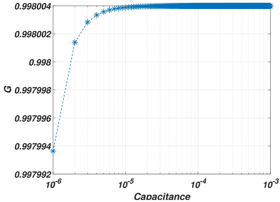
(c) Gain vs. capacitance ( $1\mu\text{F} \sim 1000\mu\text{F}$ )
