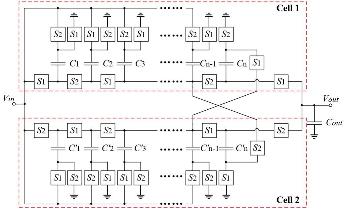
Figure 4.1: Cross-connected Dickson topology.
