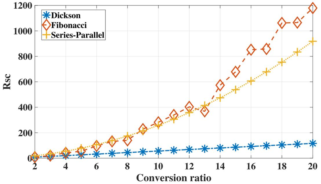
Figure 3.14:  $R_{SC}$  vs. conversion ratio.
