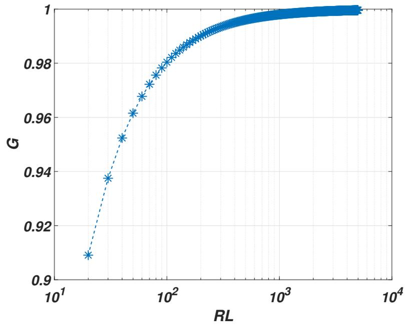
(a) Gain vs. load value ( $20\Omega \sim 5k\Omega$ )
