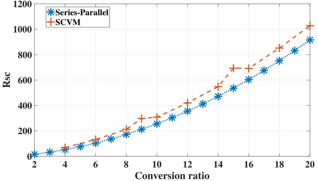
Figure 3.18:  $R_{SC}$  of SCVM and series-parallel topology at different conversion ratios.
