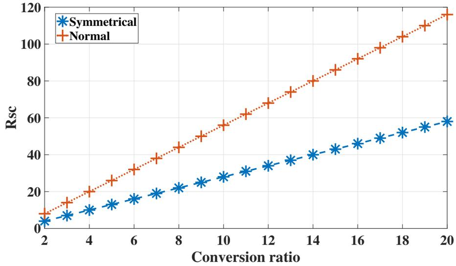
Figure 3.21:  $R_{SC}$  of symmetrical and normal Dickson topology at different conversion ratios.
