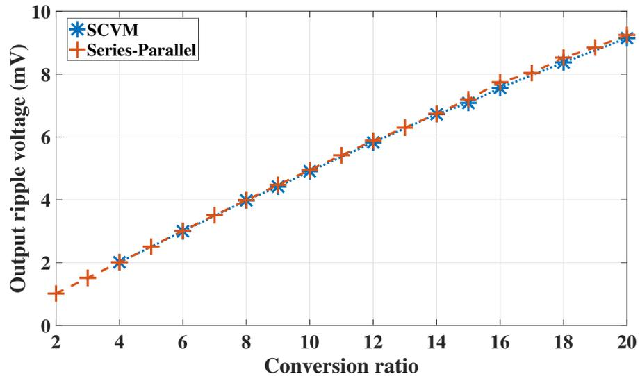
Figure 3.20: Output ripple voltages of SCVM and series-parallel topology at different conversion ratios.
