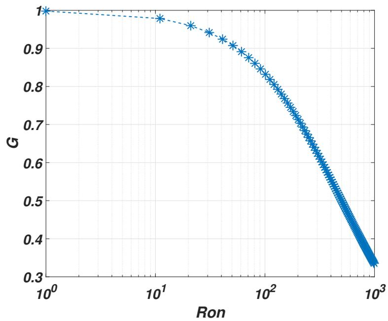
(b) Gain vs. on-resistor ( $10\Omega \sim 1k\Omega$ )
