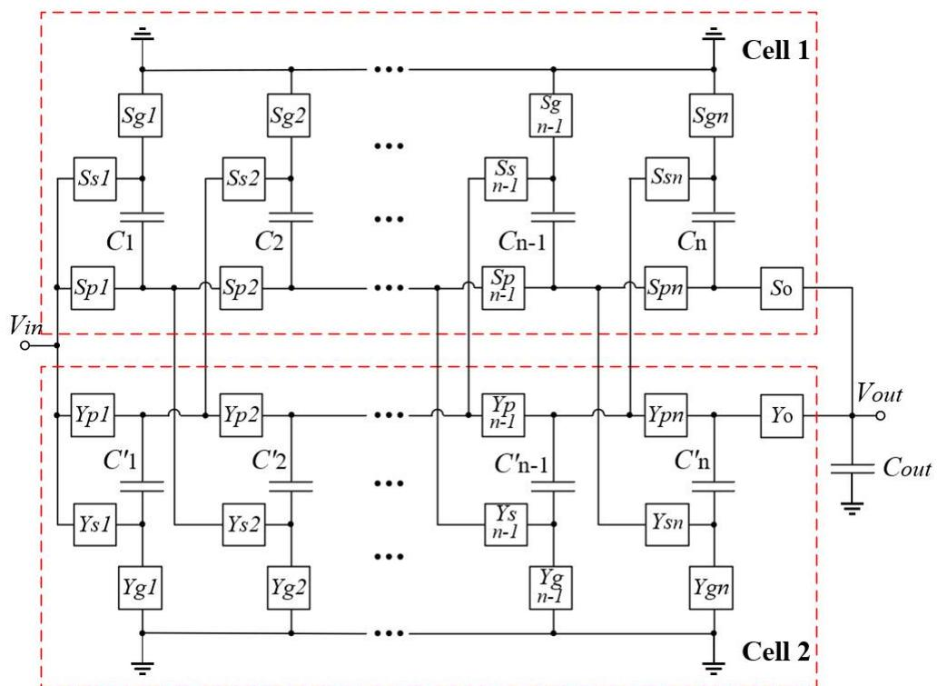
Figure 4.3: Enhanced cross-connected Fibonacci topology.
