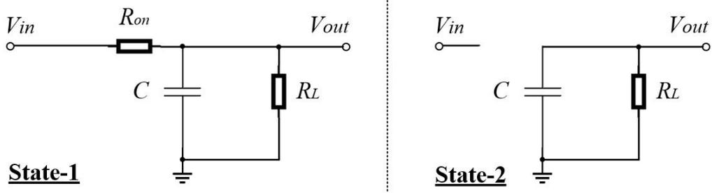
Figure 2.3: Instantaneous equivalent circuits of the simple SC DC-DC converter.
