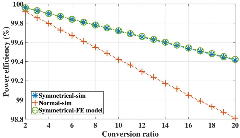
Figure 3.22: Comparison of FE model with simulation at different conversion ratios (symmetrical Dickson topology).
