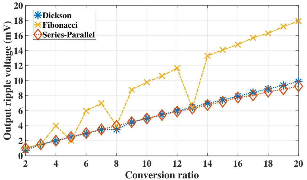
Figure 3.17: Simulated output ripple voltages of three core topologies.
