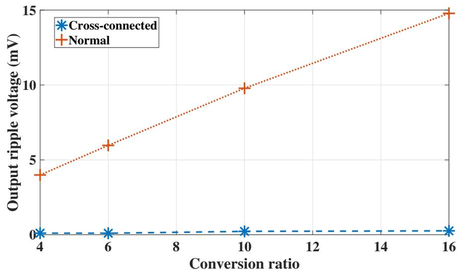
Figure 3.27: Comparison of output ripple voltages of Fibonacci topologies.
