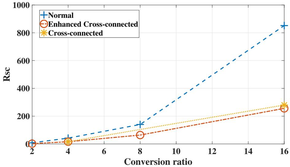
Figure 5.9: Comparison of  $R_{sc}$  of enhanced cross-connected Fibonacci topology.
