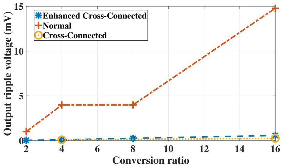
Figure 5.10: Comparison of output ripple voltages of enhanced cross-connected Fibonacci topology.
