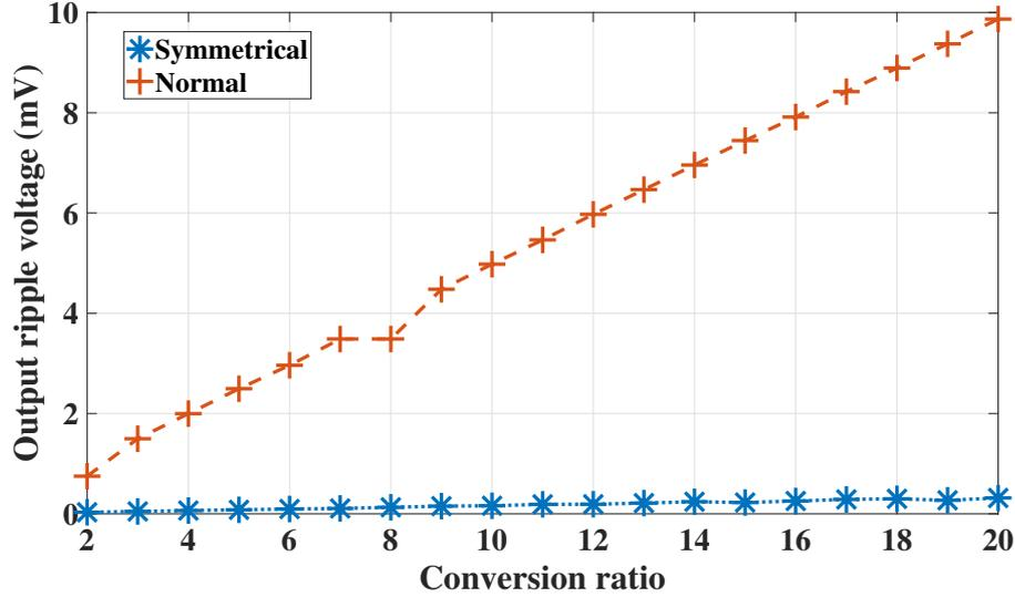
Figure 3.23: Output ripple voltages of symmetrical and normal Dickson topology at different conversion ratios.
