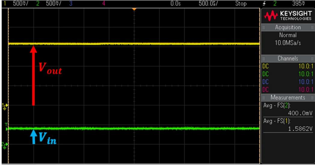
Figure 5.7: Measured output voltage of cross-connected Dickson topology.
