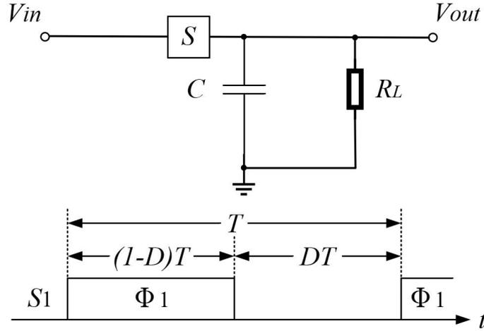
Figure 2.2: Trivial SC DC-DC converter with the conversion ratio of 1 to 1.
