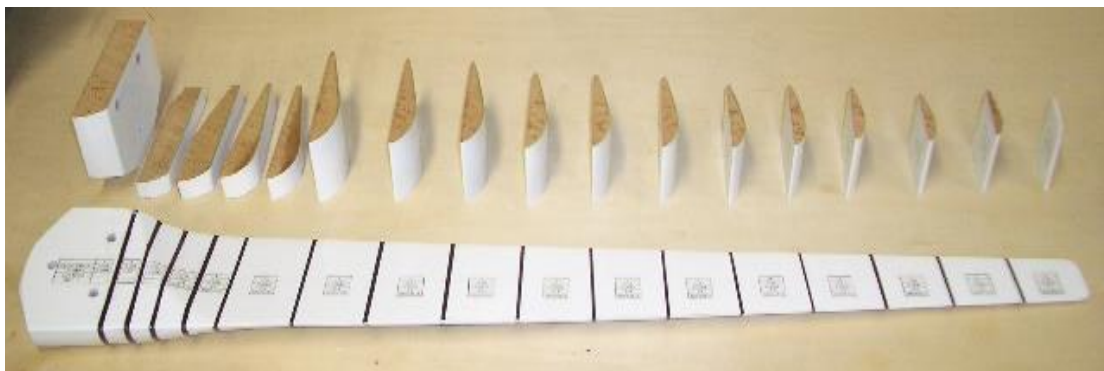
Fig. 4.3. Real wind turbine blade shape
