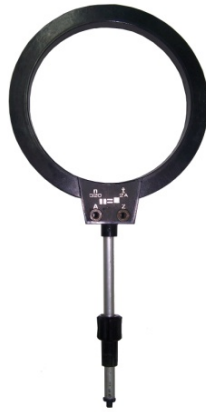
Figure 4.16: The standard Helmholtz coil of LEYBOLD DIDACTIC GMBH.
