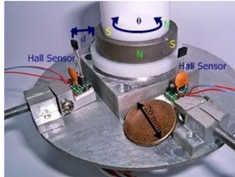
Figure 1.3: Schematic view of the angular position device containing two semi-ring shaped magnets, connected with attractive poles and double linear Hall sensor.
